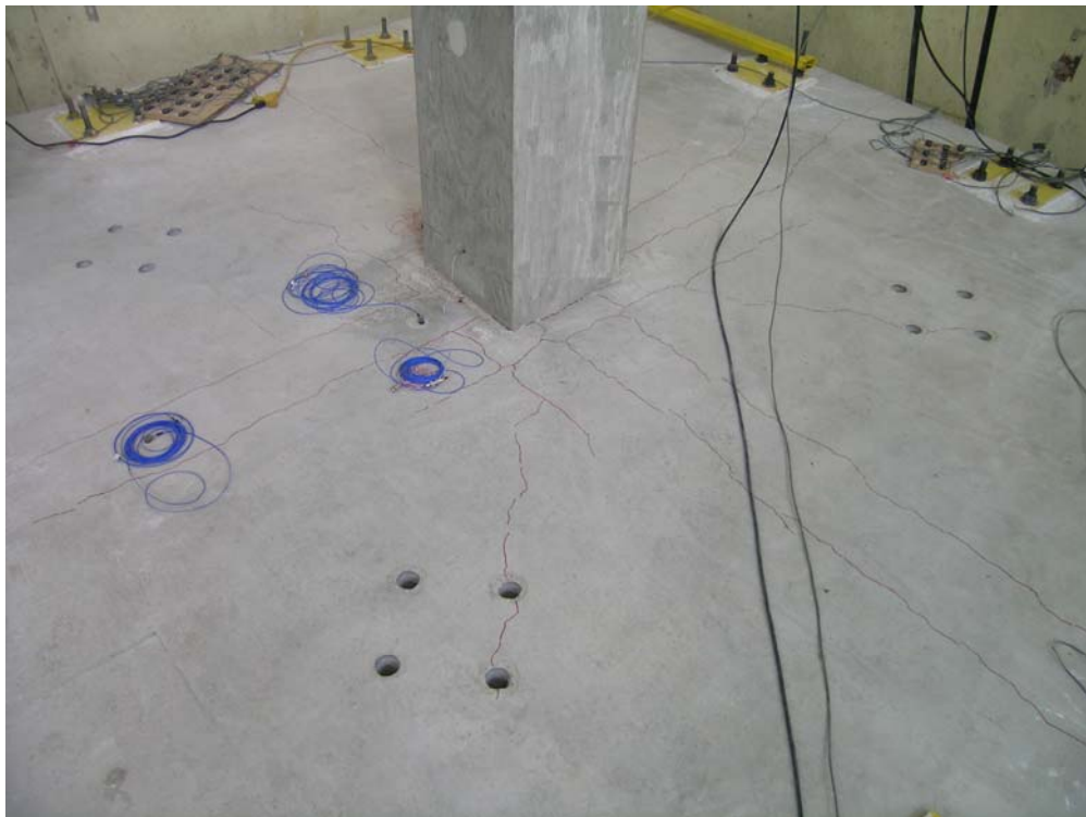
Figure 7.49 Specimen LR ST G0.5, after the application of gravity loads
