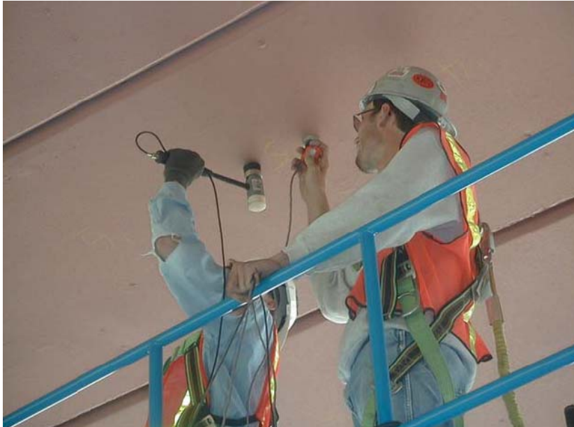
Figure 5.4 Slab Impulse Response Test (Olson, 2004)
