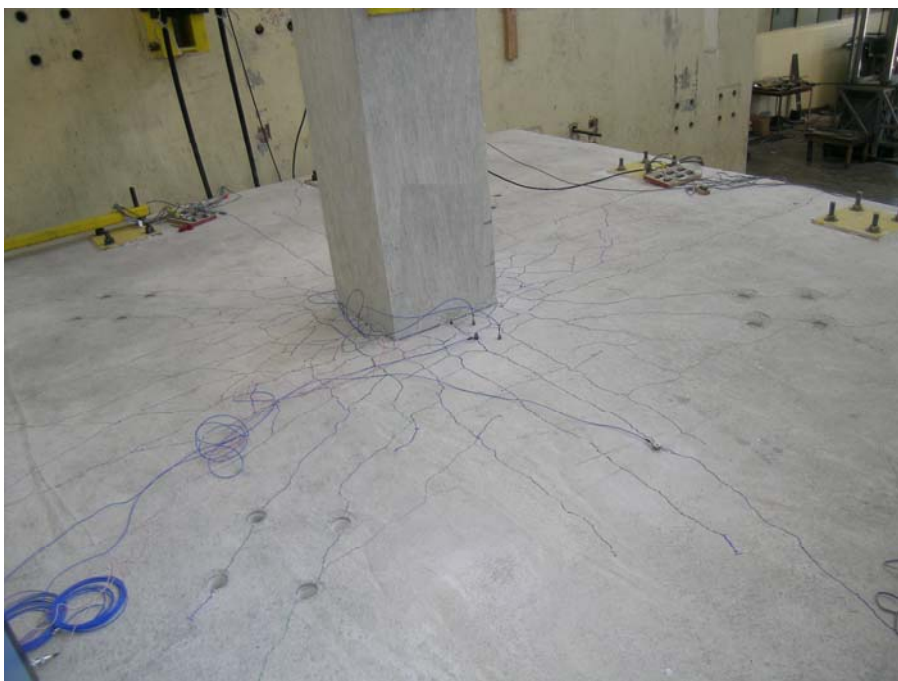
Figure 7.58 Specimen LG1.0, after application of lateral loads, at 1.25% drift
