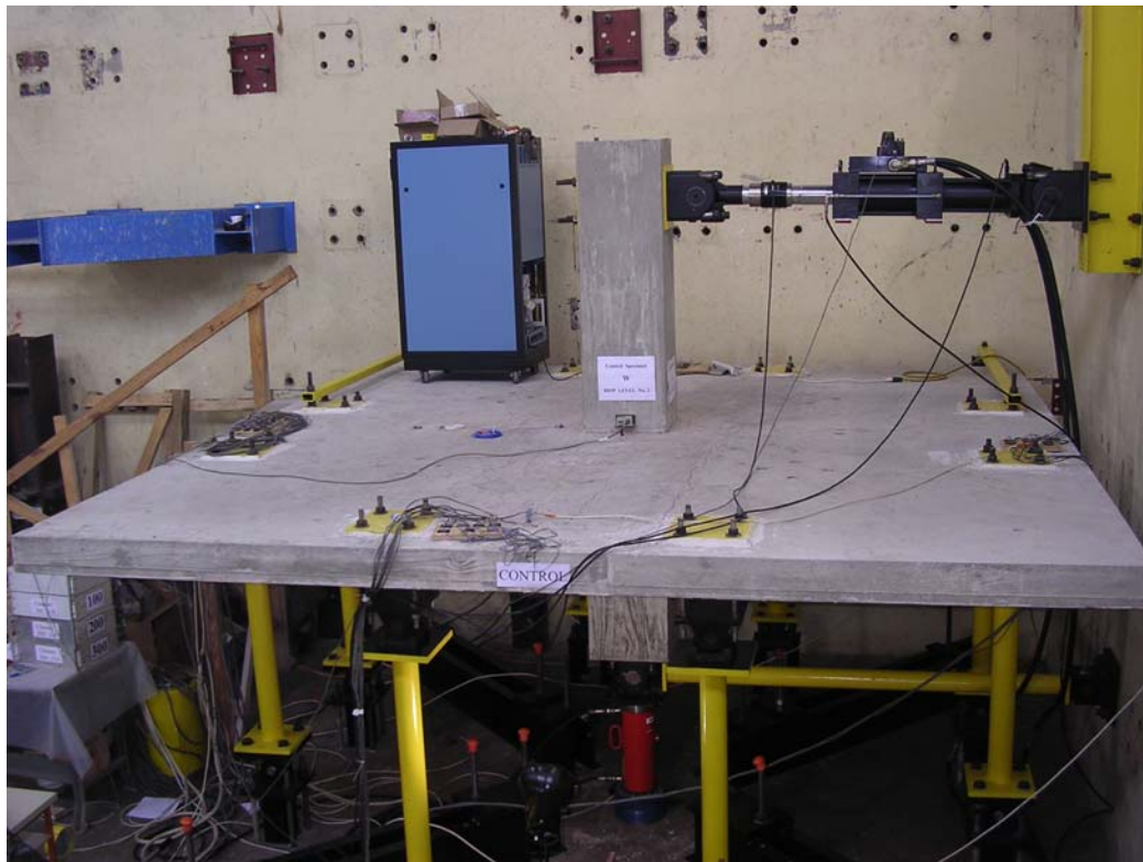
Figure 2.3 Slab-column connection tested in laboratory
