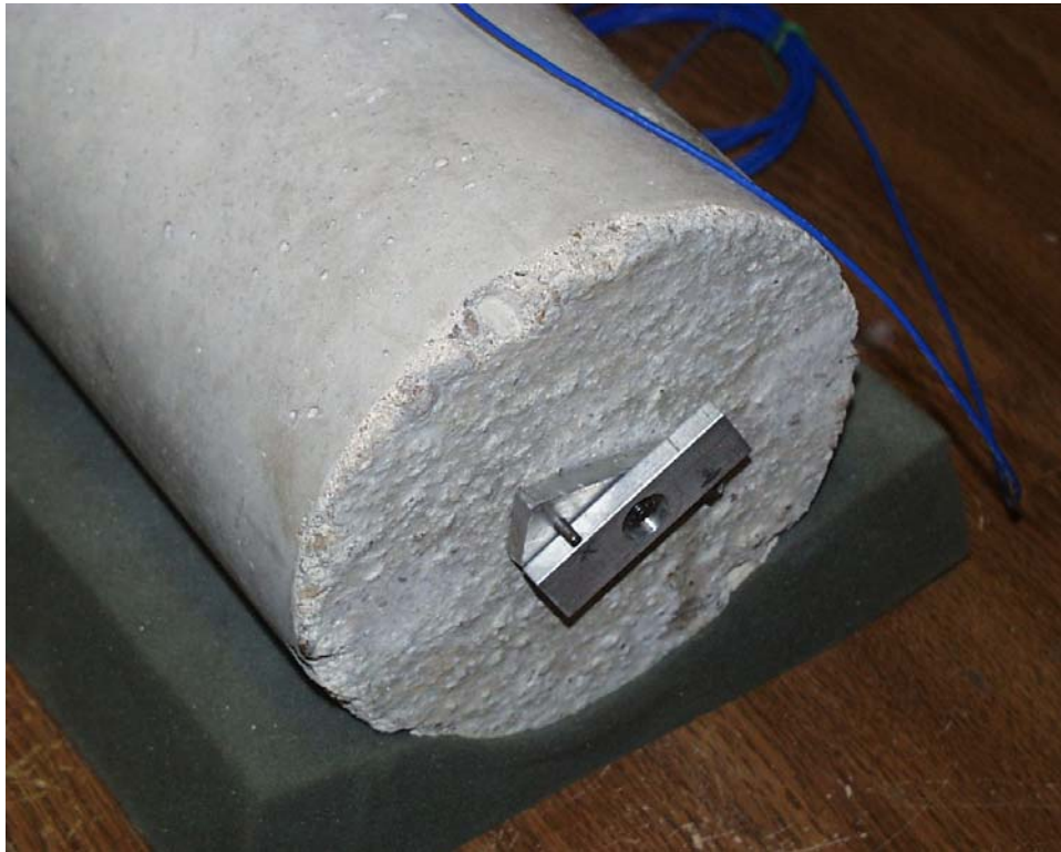
Figure B.3 Resonance Tests – Location of Impact Energy
