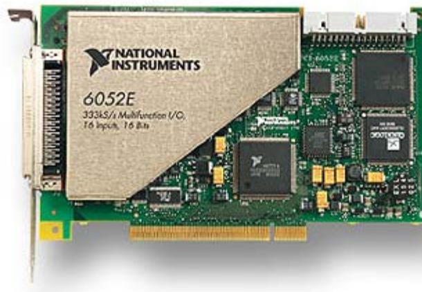
Figure 7.3 Data Acquisition Card NI PCI-6052E
