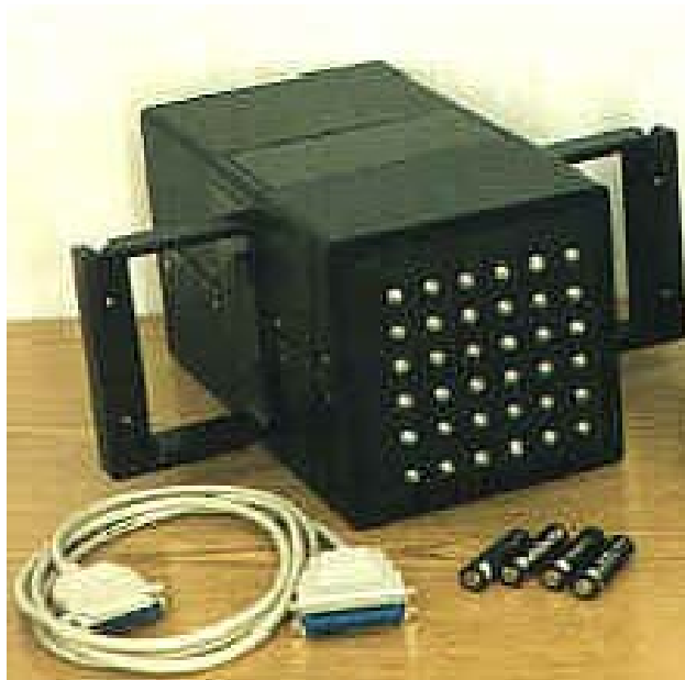
Figure 5.9 Ultrasonic phased array probe (Acoustic Control Systems, 2006)
